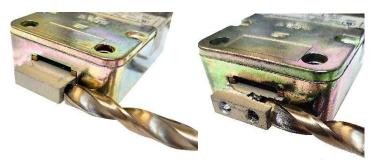
**PRO TIP)** It may be helpful to drill a 2<sup>nd</sup> smaller hole to insert a borescope into
